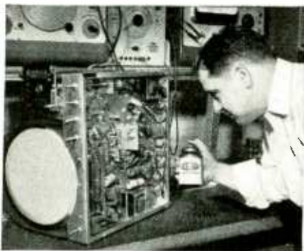
Because of its high dielectric strength, Krylon helps prevent corona. Here technician Bernard Vanella "Krylon-izes" high voltage coil and insulation, the socket of the high voltage rectifier, component parts of the rectifier circuit.
