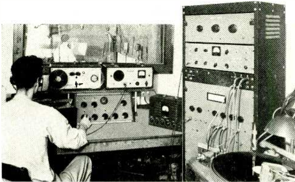
Recording-studio control room. The echo box and its controls are at the top of the rack.
